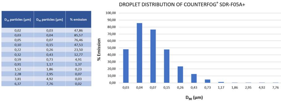
Fig. 6 Droplet distribution of COUNTERFOG® SDR-F05A+
