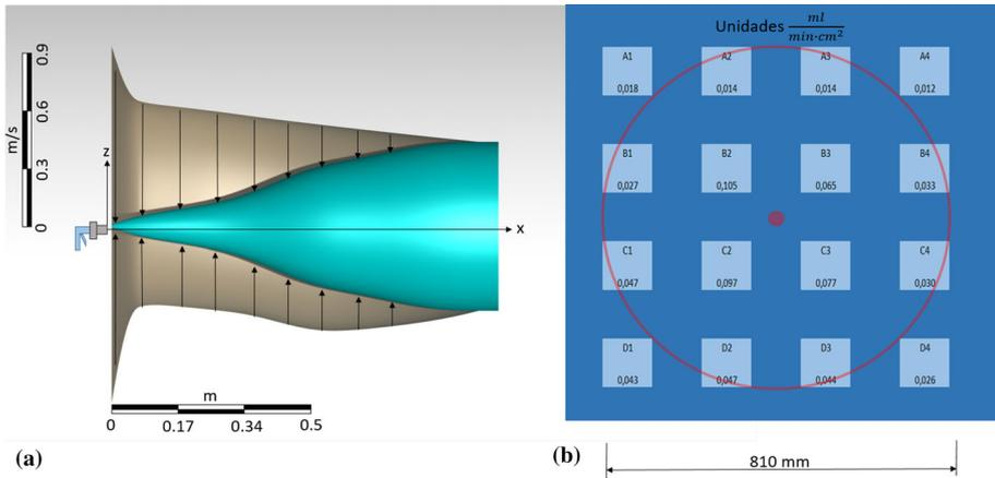
**Fig. 4** **a** Distribution of the airflow drawn in by the fog cone (m/s). **b** Distribution of the projected droplets by the fog cone at 2 m ( $ml/(min \cdot cm^2)$ )
