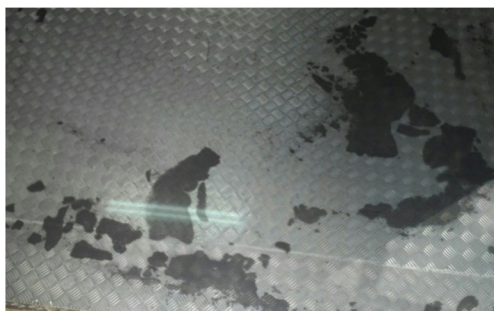
Fig. 4 Residues deposited on the floor of the camera after test
