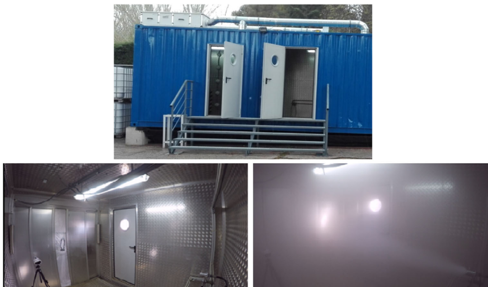
Fig. 1 Fog dynamics laboratory. Test room before and after releasing the cleaning fog
